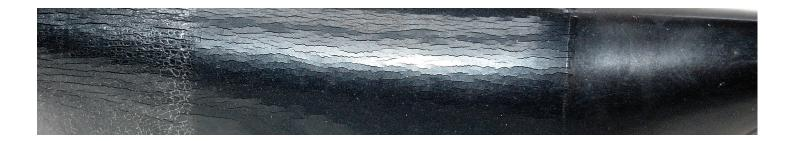
Figure 2. Neoprene pneumatic de-icing boot surface material that has been exposed to ozone. The right side was treated with a recommended treatment material.
